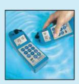
A custom LCD helps simplify calibration and operation by using annunciators and prompts to indicate various conditions.
